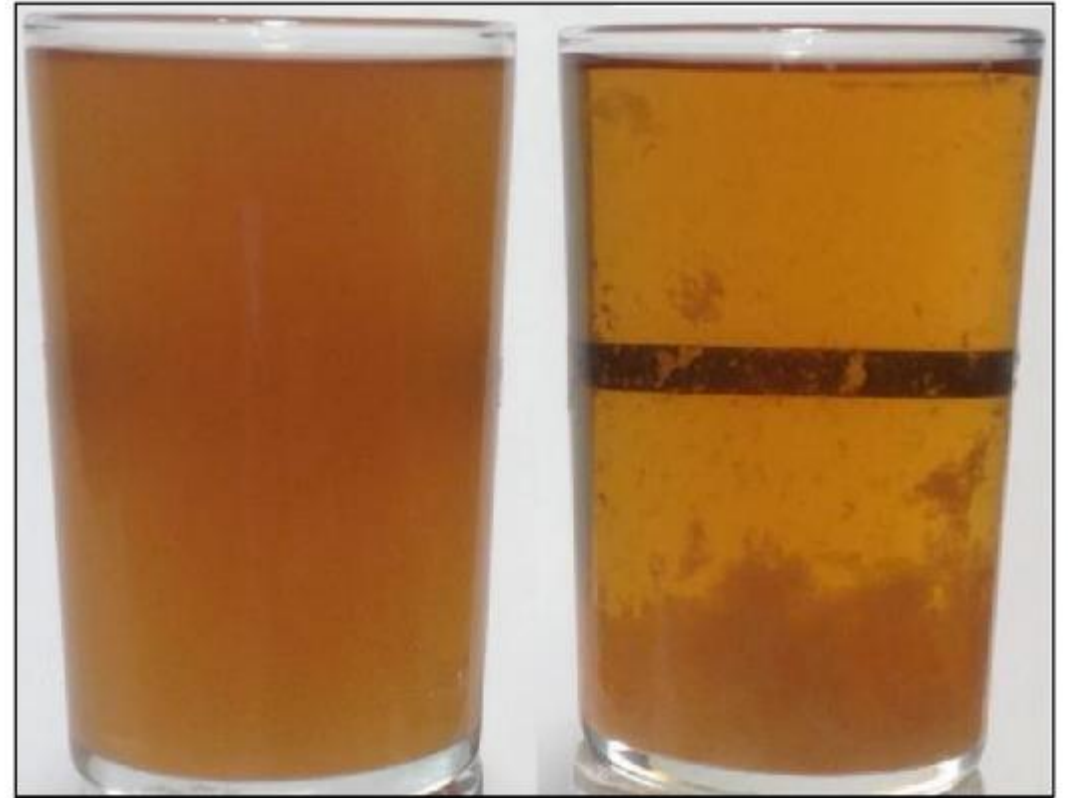
Control vs 30ppm Kettlekleer after 3 hours in 20°C wort
