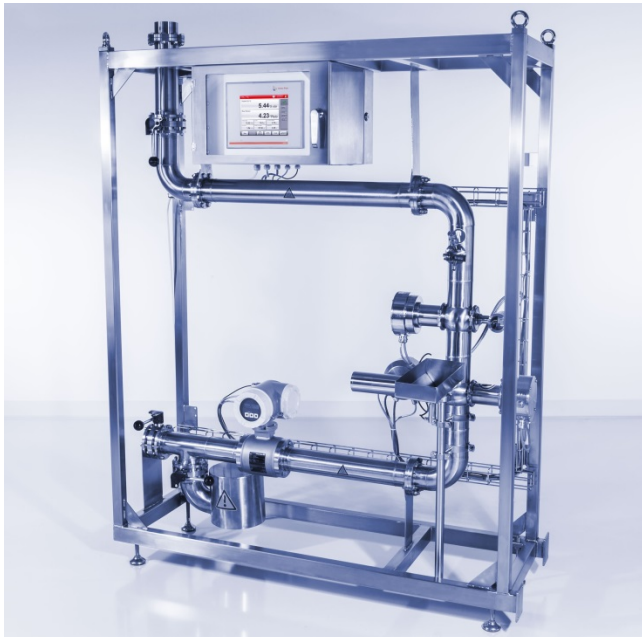
Figure 19: Beer Analysis System ready for integration
